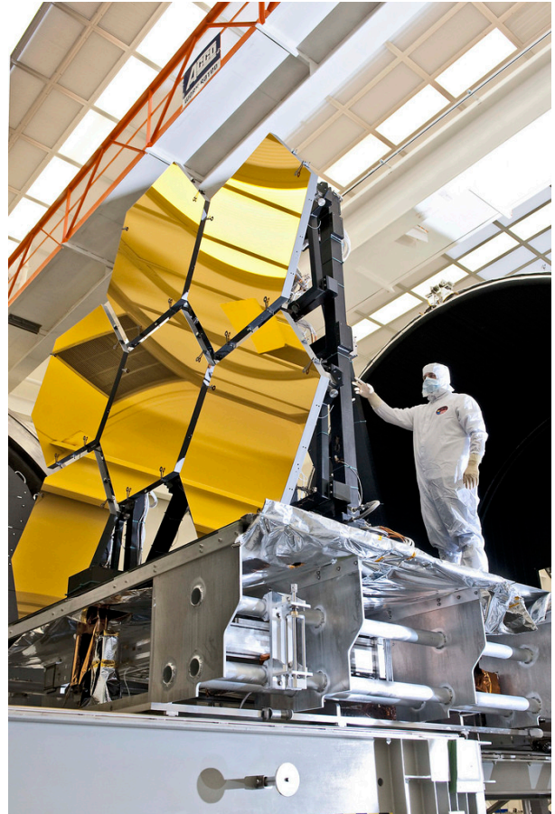
Six of the mirror segments for NASA's James Webb Space Telescope. The mirrors were built by Ball Aerospace & Technologies Corp., Boulder, Colorado
